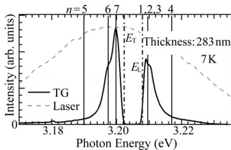
Fig. 1 TG spectrum in a CuCl thin film.  $E_T$  and  $E_L$  indicate transverse and longitudinal exciton energies of CuCl, respectively.
