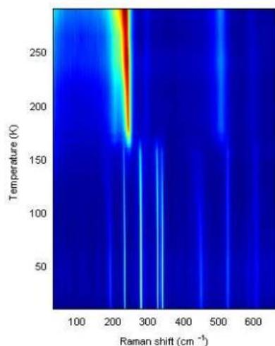
*Figure 2 Contour temperature map of  $V_2O_3$  showing a phase transition spread out around 160K with 1K resolution.*
